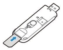
3. Insert the microSD card into the microSD card slot.
