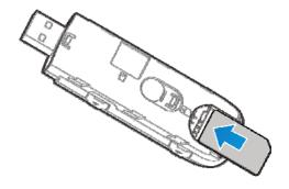
3. Insert the microSD card into the microSD card slot.
