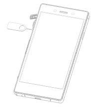
2. Pull out the card tray and place the nano-SIM card or microSDHC card on the tray, as shown. Then carefully install the tray back.
