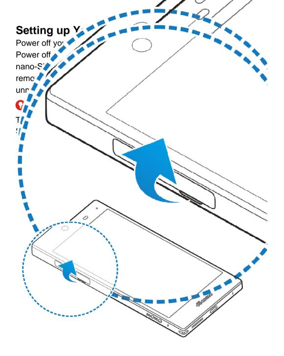
2. Insert the tip of the tray eject tool into the hole on the nano-SIM / microSDXC card tray.
