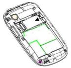
Follow the OPEN arrow to push the metal slot, and flip it up. Insert the card into the metal slot with the metal contacts facing down until it clicks to the right position.
