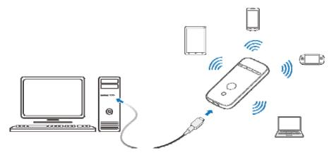
• Internet Wi-Fi Mode: Your device will connect to other WLAN device (hotspot device, wireless router, etc.) via Wi-Fi to access the Internet. The WLAN device has already connected to the Internet.
