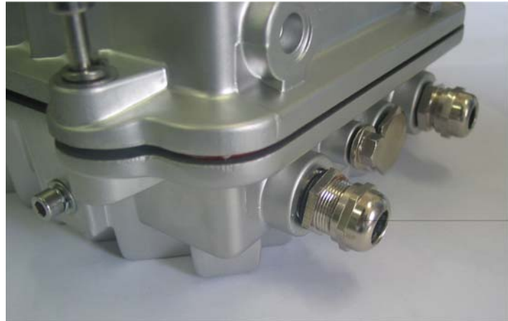
FIGURE 126 WATERPROOF END CAP INSTALLATION
