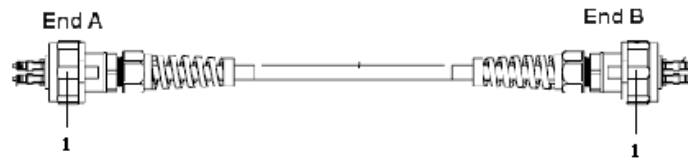
FIGURE 63 FIBER CONNECTION BETWEEN ZXSDR R8860s
