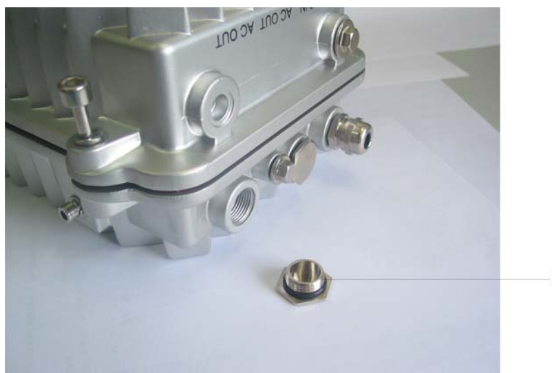
FIGURE 124 LOOSE OFF WATERPROOF END CAP
