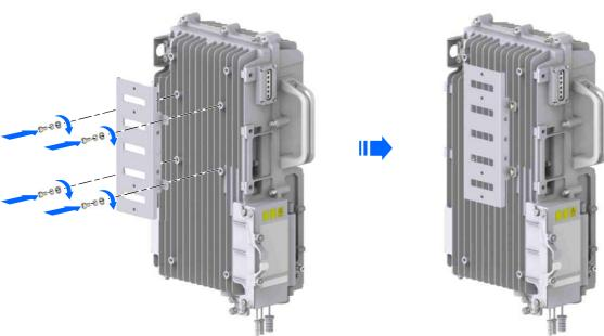
**2** Fix the lightning protection box to the mounting board.
