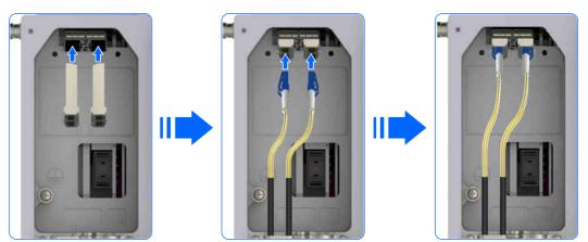
Fix the fiber to the fiber clamp in the distribution chamber.
