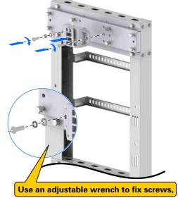
Fix the RRU to the pole fixture or mounting fixture. Use the M6 hexagonal wrench to fix the spring screws on the top of the RRU support. The L-shape support installation is completed.
