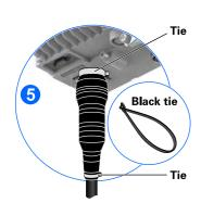
**Caution: The outermost layer of tape shall** be applied from the bottom up to avoid water penetration.
