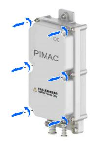
Caution: For sideor wall-mounted installation, make sure that the cover of the junction box can be opened to 90 degrees at least for DB15 easy maintenance.
