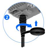
Caution: The second layer of insulation tape shall completely cover the whole feeder connector.
