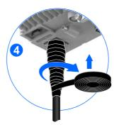
Caution: The horizontal wrapping direction refers to the direction towards which the connector is screwed tightly. Do not apply the tape in the reverse direction. The vertical wrapping direction is from the connector's bottom towards the connector.
