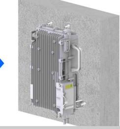
Note: Install the four expansion bolts and then mount the RRU onto the top two expansion bolts. Adjust the hole positions of the bottom two parts, align them with the expansion bolts, and then fix all the four expansion bolts.
