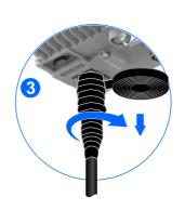
Wrap three layers of waterproof tape, as shown in Figure 2, Figure 3, and Figure 4.
