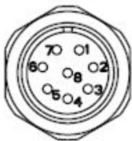
Figure 4-42 Appearance of Environment Monitor Cable
