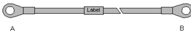
Figure 4-1 Appearance of the Protective Grounding Cable
