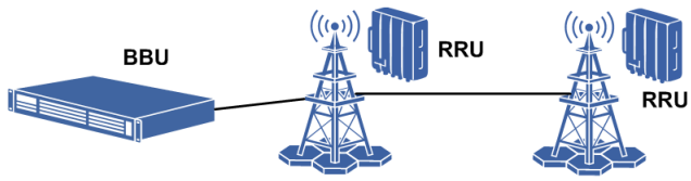
Figure 6-2 Chain Network Architecture
