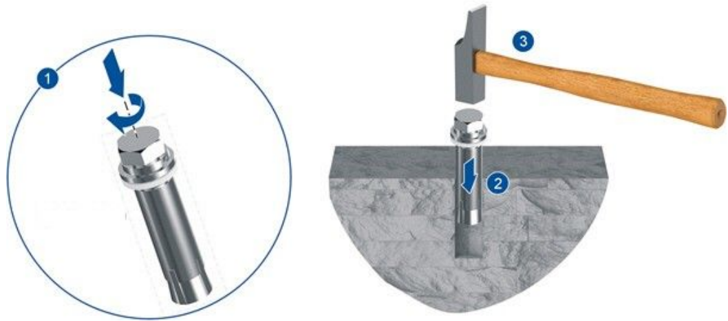
Figure 4-9 Installing an Expansion Bolt 2
