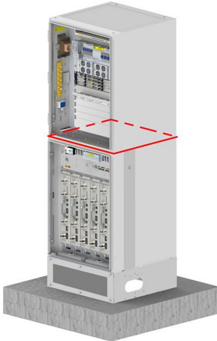
Figure 4-25 Sealing Apertures of Stacked Cabinets by Using Seamgum
