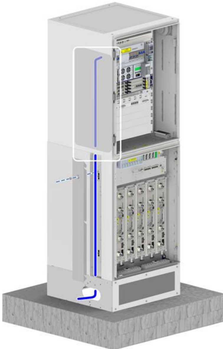
Figure 7-1 External Cable Routing of the BC8910A Cabinet
