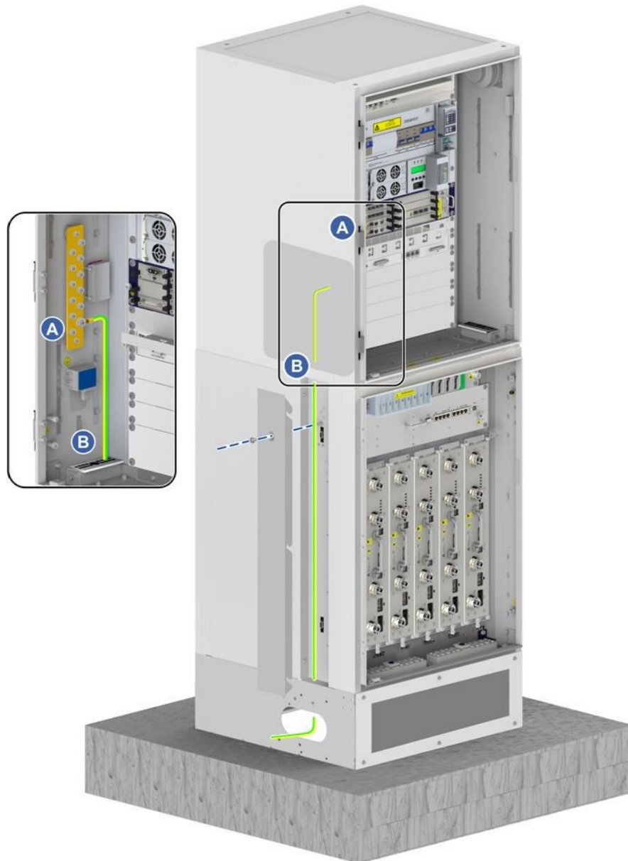
Figure 7-12 Fixing the Grounding Cable to the Copper Grounding Bar
