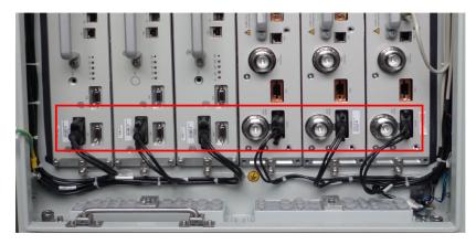
Figure 5-8 Power Cable Connecting the RSU
