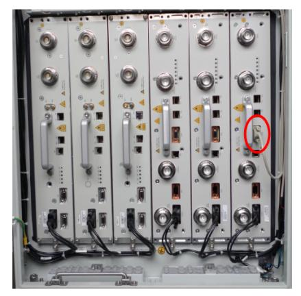
Figure 5-10 Installing the RSU Monitoring Cable
