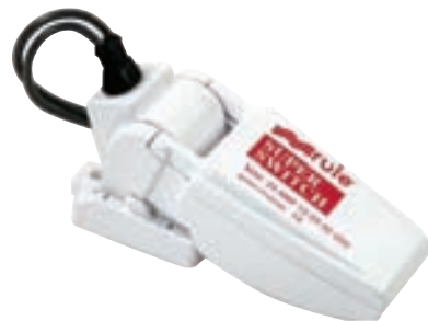
37A SuperSwitch™ float switch, 2¼" x 5" x 2" (57 x 127 x 51mm), 12-24-32v DC, fuse 20amp (12v), 10amp (24v), 6.5 amp (32v). 37FA SuperSwitch™ float switch with fuse holder.
