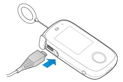
Plug the AC adapter into an electrical outlet. Fully charging a battery may take up to three hours.
