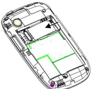
3. Follow the OPEN arrow to push the metal slot, and flip it up. Insert the memory card into the metal slot with the metal contacts facing down until it clicks to the right position. Flip the metal slot back and follow the LOCK
