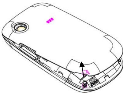
2. Hold the SIM card with the cut corner oriented as shown and slip it into the card holder.
