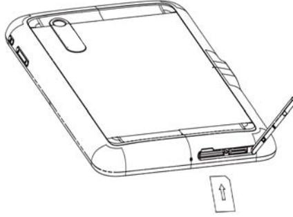
2. Insert your memory card into the memory card slot. There is a diagram showing the correct orientation of the card printed above the memory card slot.
