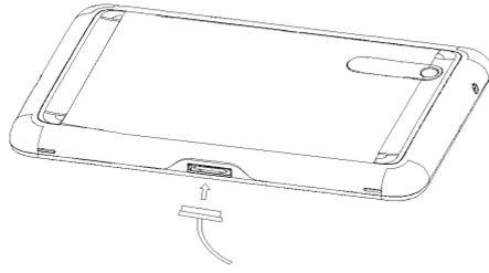
3. Disconnect the charger when the battery is fully charged.
