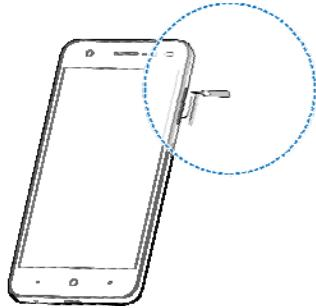
2. Pull out the nano-SIM card tray or microSDHC card tray and place the nano-SIM card or microSDHC card on the tray, as shown. Then carefully install the tray back.
