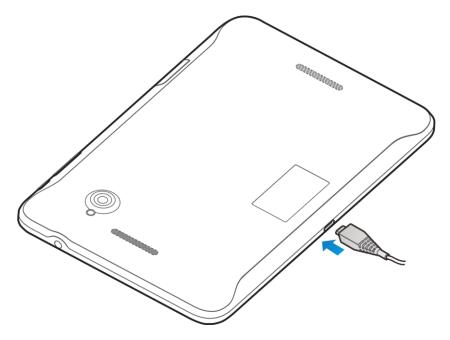
Plug the USB cable into the AC adapter, and then plug the AC adapter into an electrical outlet. Fully charging a battery may take up to three hours.
