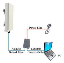
To obtain the best radio signal level and connection quality, the CPE antenna should be aimed towards the best eNB or BS directly. To search for the best eNB direction, the user can rotate the CPE slowly and tilte CPE slightly to find the best signal direction. The CPE radio signal strength level can be observed from the RF LEDs mounted on the lower panel as shown below. The more LEDs on, the better the signal strength.
