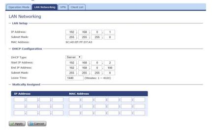
The LAN setting allows user to specify the DHCP server setting for the LAN devices including the pool address, IP and MAC binging and whether DHCP server should be enabled.
