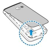
Hold the microSDXC card with the cut corner oriented as shown and slip it into the card slot.
