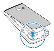
Insert the battery. Make sure the connectors on the battery go into the battery compartment first and align with the connectors in it. Gently push down on the battery until it clicks into place.
