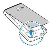
Slide the micro-SIM card into the card holder in the battery compartment.
