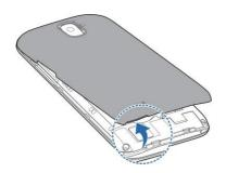
Hold the microSDHC card with the cut corner oriented as shown and slip it into the card slot.
