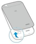
Hold the micro-SIM card with the cut corner oriented as shown and slip it into the card holder.
