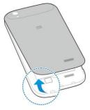
Insert the microSDHC card into the slot with the golden contacts on the card facing down.
