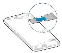
**NOTE:** Some applications may require a microSDHC card to work normally or may store certain data on it. Therefore, it is recommended that you keep a microSDHC card installed and not remove or replace it randomly.
