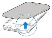
2. Hold the micro-SIM card with the cut corner oriented as shown and slip it into the card holder.
