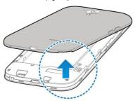
2. Hold the micro-SIM card with the cut corner oriented as shown and slip it into the card holder.
