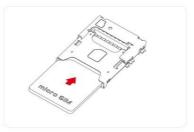
Insert the memory card into the metal slot with the metal contacts facing down until it clicks to the right position.
