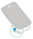
2. Hold the nano-SIM card with the cut corner oriented as shown and slip it into the card holder.
