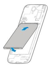
Align the back cover with the back of the phone and press the cover back into place. Ensure that all the tabs are secure and there are no gaps around the cover.
