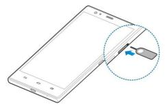
Pull out the tray and place the card on the tray, as shown. Then carefully install the tray back.
