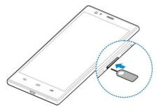
Pull out the micro-UIM card tray and place the micro-UIM card on the tray, as shown. Then carefully install the tray back.
