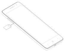
Pull out the card tray and place the nano-SIM card (right) /microSDXC card (left) facing down on the tray. Gently slide the card tray in until it clicks into place.
