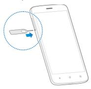
Place the nano-SIM/microSDXC card on the tray with the gold-colored contacts facing down. Then carefully slide the tray back into place.
