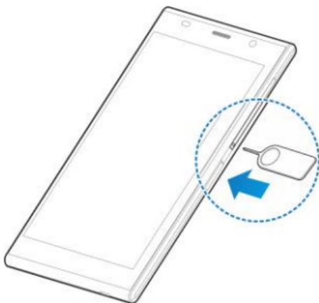
2. Pull out the micro-SIM card tray and place the micro-SIM card on the trays as shown. Then carefully install the tray back.
