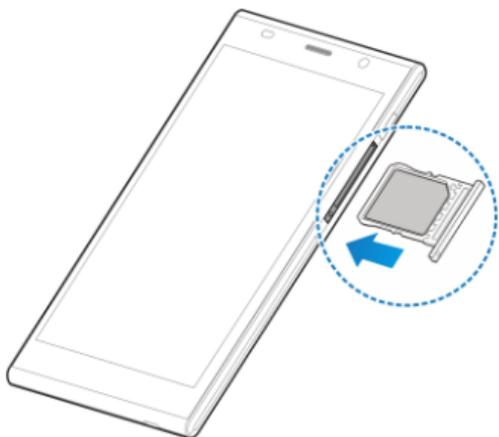
3. Insert the tip of the tray eject tool into the hole on the microSDHC card tray.
