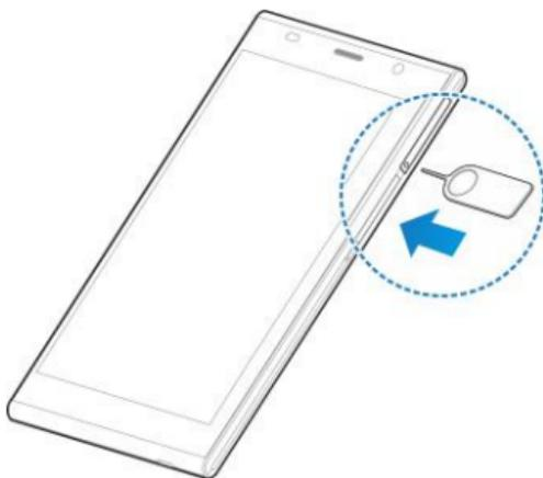
4. Pull out the tray and place the card on the tray as shown. Then carefully install the tray back.
