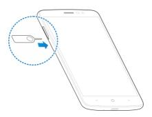
Pull out the card tray and place the nano-SIM card on the tray, as shown. Carefully slide the tray back into place.
