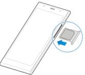
Insert the tip of the tray eject tool into the hole on the microSDHC card tray.
