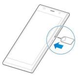
Pull out the micro-SIM card tray and place the micro-SIM card on the trays as shown. Then carefully install the tray back.
