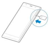
Pull out the tray and place the card on the tray as shown.
