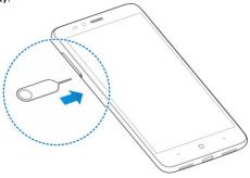
Pull out the card tray and place the nano-SIM card (right) /microSDXC card (left) facing down on the tray. Gently slide the card tray in until it clicks into place.
