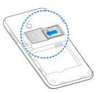
Insert the battery by aligning the metal contacts on the battery with the metal contacts in the battery compartment. Gently push down on the battery until it clicks into place.
