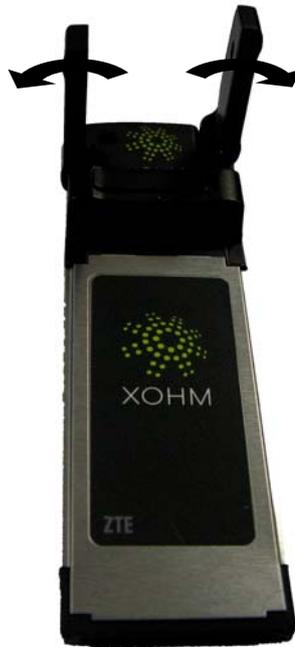
**Step 2:** Connect the modem to your PC. Ensure that it is tightly inserted.
