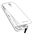
2. Hold the SIM card with its cut corner oriented as shown and slip it into the card holder.
