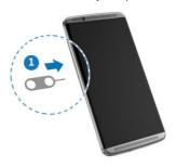
Place the nano-SIM/microSDHC card (not included) on the tray with the gold-colored contacts facing down, and then carefully slide the tray back into place.
