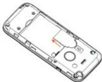
Pull out the SIM card
