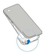
Install the nano-SIM card and the microSDXC card as 2. shown
