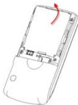
Pull up the battery from here
