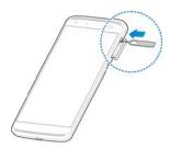
2. Pull out the nano-UIM / nano-SIM card tray or microSDHC card tray and place the nano-UIM / nano-SIM card or microSDHC card on the tray, as shown. Then carefully install the tray back.
