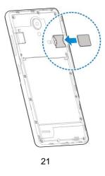
3. Hold your microSDXC card with the metal contacts facing down and slide it into the microSDXC card slot.
