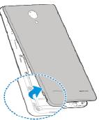
2. Hold the nano-SIM card with their cut corner oriented as shown and slip it into the card holder.
