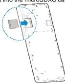
4. Insert the battery by aligning the golden contacts on the battery and those in the battery compartment. Gently push down on the battery until it clicks into place.
