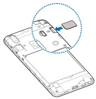
3. Hold your microSDXC card with the metal contacts facing down and slide it into the microSDXC card slot.
