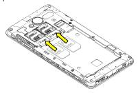
3. Insert the memory card into the card slot with the metal contacts facing down until it inserts to the right position.
