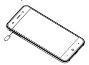
2. Pull out the nano-SIM card tray and place the nano-SIM cards on the tray, as shown. Then carefully install the tray back.
